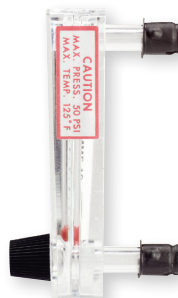
Model MMF mounts easily from front of panel. Drill two 9/32" or 5/16" dia. holes in panel on 2-1/16" centers. Insert mounting connector spuds. From rear, slide on the two spring retainers (furnished) and push on rubber or plastic tubing.
