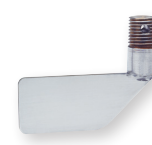
PDL-4 Minimum bulk density of 70 lb/ft³ (1122 kg/m³). Fits through 1-1/4" coupling eliminating the need for a mounting flange.
