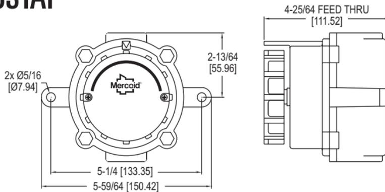
Explosion-proof, heavy duty, the **MODEL 862E** Thermostat is designed for hazardous-location temperature control of heating, cooling, or ventilation systems and features an adjustable set point knob for easy and convenient setpoint adjustment.
