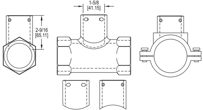
The **SERIES EFF** Fittings & Tees is to be used with the Series EFS2 Insertion Electromagnetic Flow Sensors. The Series EFF allows for accurate sensor insertion of the Series EFF in a wide range of pipe sizes. These fittings and tees are available in bronze, 304 SS, 316 SS, and PVC, further expanding application prospects.
