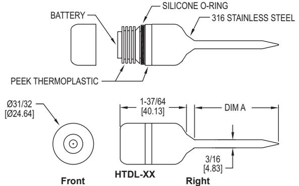
The **MODEL HTDL-20/30** is a high temperature data logger that can measure temperatures up to 500°F (260°C) and record up to 32,700 measurements.
