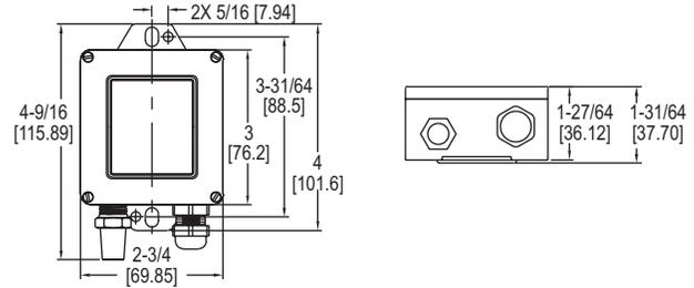
The compact **SERIES WHT** Humidity/Temperature Transmitter is designed to withstand the elements. A removable sintered filter protects the polymer capacitance sensor from solid objects that may come in contact with the transmitter. The transmitter is available with 4 to 20 mA or 0 to 10 VDC output signals for both temperature and humidity. This transmitter is ideal for measuring outside air temperature and humidity levels for air handling economizer applications.
