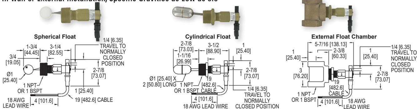
The **SERIES L10 FloTECT®** Mini-Size Float Switches is a series of economical, compact liquid level floats. It is offered in brass or 303 SS bodies and external tees as well as polypropylene or 304 SS floats with 1" NPT male threads, for direct side mounting through a half coupling, or with factory installed tee for external mounting. This series can be used in liquids with specific gravities as low as 0.5.
