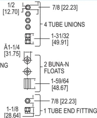
The **MODEL F7-MLK** Multi-Level Switch Kit provides a customized level system to suit specific application requirements. The F7-MLK Multi-Level Switch Kit contains all the components necessary for the design and fabrication of a 1 or 2 station level switch for pipe plug mounting.
