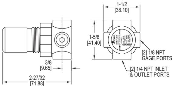
The **SERIES MPR** Miniature Pressure Regulators are compact units that provide low cost, high performance pressure regulation of compressed air or air/water. The low torque, non-rising adjustment knob with locking capability provides easy and precise adjustment. Models for use with air are self relieving. Models for air/water are non-relieving.
