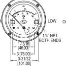
4X ø3/16 [ø5.16] EQUALLY SPACED ON A ø5-5/8 [ø142.85] BOLT CIRCLE ø5-9/32 [ø133.97] PANEL CUTOUT
