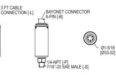
The **SERIES 644** High Accuracy Pressure Transmitter is a robust transmitter designed for high accuracy pressure applications. Boasting an accuracy of  $\pm 0.05\%$  FS RSS (< $\pm 0.25\%$  TEB), the 644 is intended for precise measurements in the critical applications.
