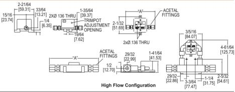
The **SERIES TFP-GV** Gas Flowmeters utilize a turbine wheel and electro-optical detection to convert flow rates into a linear 0 to 5 VDC output signal for recording and data logging. A power adapter or mating cable assembly is required for operation.
