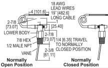
The SERIES V10 Flotect® Mini-Size Flow Switches is designed to provide inexpensive. reliable monitoring of the presence or absence of flow in a system. This series is available for field installation in pipelines from 1/2 to 2" diameter and available in brass or 303 SS body.
