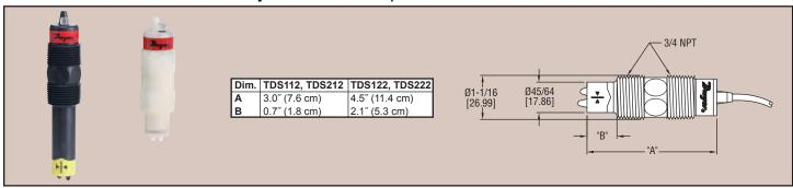
The Series TDS Thermal Dispersion Flow Switch offers solid state flow detection of non-coating liquids for pump and process protection. SPDT output allows for interfacing with remote PLC or relay control device. The adjustable switch point is factory calibrated at 0.2 fps with LED indication of flow and calibration status. Units feature selectable NO or NC operation and are not damaged by overranging flow velocities.
