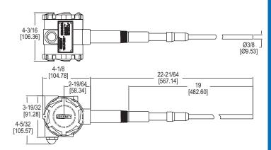
The SERIES CLS2 Capacitive Level Switches is a capacitive technology level switch which can be used for liquids, powders and bulk materials. It is offered with PVDF and 316 SS wetted material, weatherproof enclosure, DPDT output and a variety of process connections.
