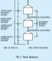
The most versatile liquid level controls in our line, displacer controls can be used to trigger alarms, provide shutdown or operate pumps.
