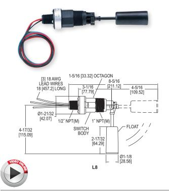
The MODEL L8 Flotect® Liquid Level Float Switches is a float switch constructed of polyphenylene sulfide, Ceramic 8 and 316 SS. This liquid level switch provides accurate set point control of liquids with specific gravities as low as 0.6.
