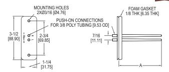
The SERIES PAFS-1000 Averaging Flow Sensor is ideal for sensing velocity pressure in the inlet section of variable air volume terminal units and fan terminal units.
