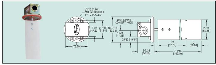
**The Model 530 air flow switch** provides excellent sensitivity and reliability at a very reasonable price. Quality features include a rugged die cast body, stainless steel vane and SPDT snap switch. Unit is field adjustable from 400-1600 FPM. Mounting is fast and simple, with only two screws needed. Vane fits 6 in. or larger ducts.
