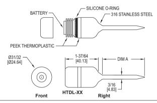
The MODEL HTDL-20/30 is a high temperature data logger that can measure temperatures up to 500°F (260°C) and record up to 32,700 measurements.
