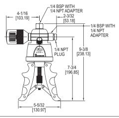
The SERIES HCHP Hydraulic Calibration Hand Pump utilizes a fully adjustable stroke control that allows for quick priming, easy pumping, and fast pressure generation up to 10,000 psi (700 bar). The ergonomically engineered handles provide extra comfort, while the triple filtration system ensures pump operation in spite of dirty conditions.
