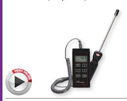
The MODEL 485B Thermo-Hygrometer is a versatile, compact, handheld instrument for measuring percentage of relative humidity and temperature in °F or °C. Dew point and wet bulb temperatures are derived from the relative humidity and temperature measurements and are displayed on the LCD.
