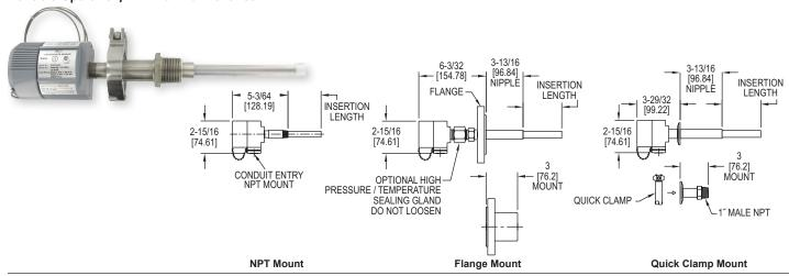
The SERIES PMS Particulate Sensor employs a field-proven combination of passiveinduction and protected-probe technologies. As particles flow near and around the probe, the signal is processed into an absolute output that can be sent to a Series DPM Particulate Monitor. Protective layers over the probe work in combination with induction-sensing to ensure reliable operation with all types of particulate including moist powders and highly conductive dusts.
