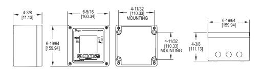
The SERIES DPM Particulate Monitor and Series PMS Particulate Sensor combine to provide a basic baghouse and cartridge filter leak detector designed for general maintenance planning and process protection. Leakage is gauged in real-time, on-thespot, without prior baseline data and without signal tuning and displayed on the digital readout in a bar graph and an absolute digital readout. An alarm point can be set by simply moving an indicator up and down the gauge with the key pad.
