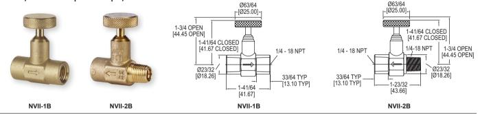
The **MODEL NVII** Needle Valve provides easy flow regulation in all applications, including shut off and throttling for pressure gages and instruments. With a one piece, hot forged brass body construction, years of maintenance-free service can be expected. The Model NVII, with its tamper-proof design and blowout-proof stem, provides excellent performance and reliability.
