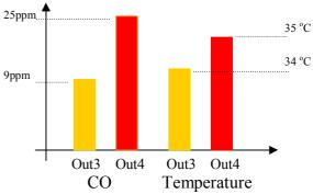
The CO level or temperature, whichever reaches the preset trip point activates the relay contacts. 9ppm CO or 34 °C in temperature will trigger relay contact at Out3; while 25ppm CO or 35 °C temperature will trigger second relay contact at Out4. [CP-13 Singapore]
