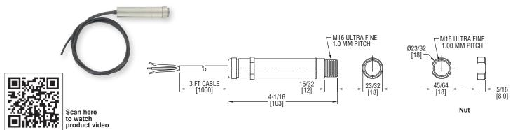
The **SERIES ILA** Non-Contact Sensors, measure temperatures from 32 to 932°F (0 to 500°C) and provide a linear 4 to 20 mA or thermocouple output. The 2-wire signal is compatible with almost any indicator, controller, recorder, data logger, etc., without the need for special interfacing or signal conditioning. They are suitable for most materials such as food, paper, textiles, plastics, leather, tobacco, pharmaceuticals, chemicals, rubber, coal, and asphalt.
