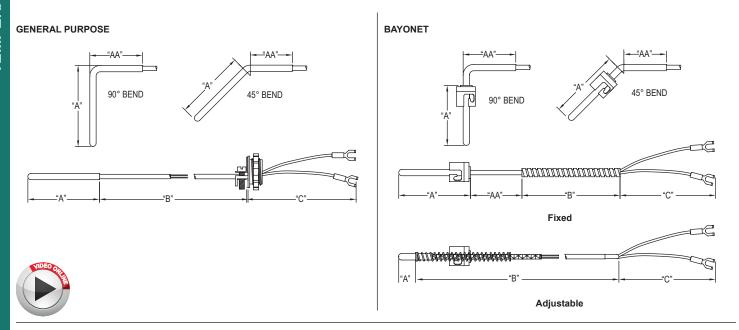
SERIES 4 & 5 General Purpose Type RTD and Thermocouple tip temperatures can be as high as 842°F (450°C) for fiberglass insulated wire, and 392°F (200°C) for FEP insulated wire. Models can be specified with lead wires or head assembly construction. For higher temperatures see the Series R & 8 Mineral Insulated Probes.
